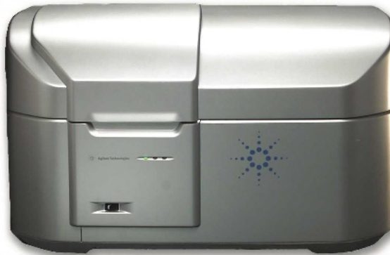
Agilent's DNA microscanner has a resolution of 2 micrometres.
